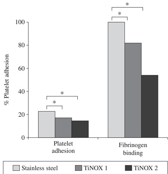
Figure 2.—Platelet adhesion and fibrinogen binding with the titanium-nitride-oxide-coated bioactive stent *versus* a 316L stainless steel stent of a similar design in a porcine model. \* means  $P < 0.05$ .
