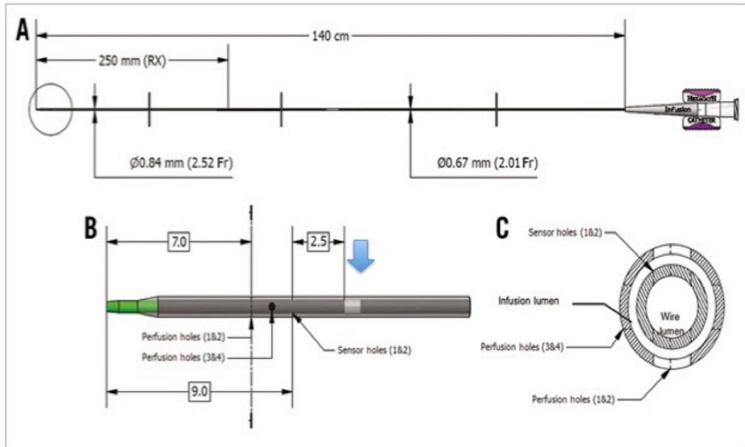
RayFlow infusion catheter. A) Schematic drawing and dimensions of the design of the infusion catheter. B) Close-up of the tip (indicated in the circle in A), highlighting the four infusion holes and the two sensor holes. The blue arrow indicates the radiopaque marker of the catheter. C) The cross-section of the catheter tip at the most distal infusion holes (1 & 2), as indicated by the dashed line in B. The lumen for the guidewire and for the infusion as indicated.
